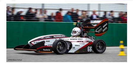
The fully electrically powered 4WD race car from "Starkstrom Augsburg e.V."provides it's live telemetry data online. Therefore, the LTE network is used and not the at the events of formula student often overloaded 2,4 GHz WiFi.
